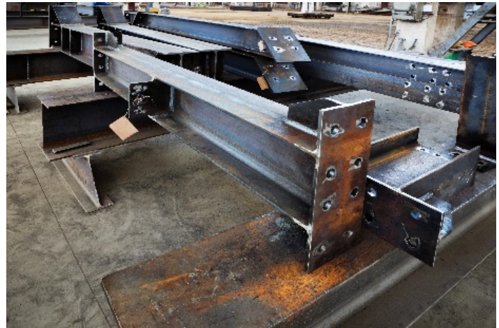
Unprotected Rusted Beam
