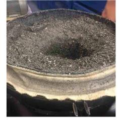
20 microns, it should be replaced with a larger mesh size to avoid clogging and ensure antifoam additives are not being removed.
