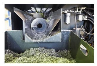
During a metalworking operation, chips are continuously being produced. These can build up on the workspace, in the sump and in filters (as demonstrated in the picture to the left). It is essential these chips are removed from the workspace and not allowed to build-up in the machine. Excess chips give the fluid and foam more surface area to cling to which prevents the foam from breaking and properly dispersing.
